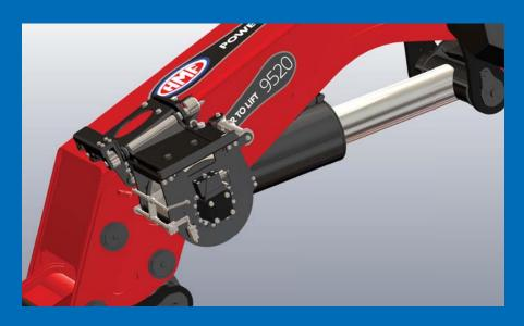
Now it is even easier to work with a hoist. The wire rope runs in automatically when you fold up the crane.
