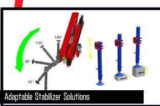
The crane's stabilizer legs are robust, easy to handle and require minimum space. You can choose between fixed stabilizer legs or manual swing-up stabilizer legs (45°, 90°, 135°, 180°) with or without gas spring. The stabilizer cylinder is adjustable by +/- 200 mm in height, with full stroke.
