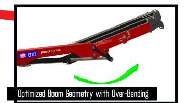
The boom system is equipped with single Power Plus link arm system on the jib, allowing a maximum load moment with stretched boom system. It is additionally fitted with a "genuine" HMF over-bending of 15° which means that the crane is capable of lifting the maximum capacity in the maximum over-bending position.
