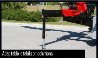
The stabilizer legs of the crane are to ensure stability - however they still have to be sturdy, easy to handle and must not take up too much space when not in use. Therefore you can choose between fixed stabilizer legs, manual swing-up stabilizer legs to 180° with gas spring or fully hydraulic swing-up stabilizer legs to 180°. Stabilizer beams can be freely selected as hydraulically extensible or manually extensible, also in connection with the sophisticated EVS stability monitoring.
